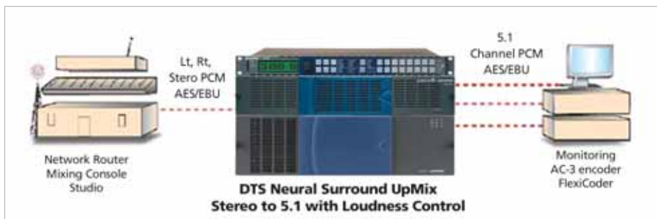
DTS Neural Surround UpMix is commonly used for audio monitoring, and in production studios and DTV facilities.
