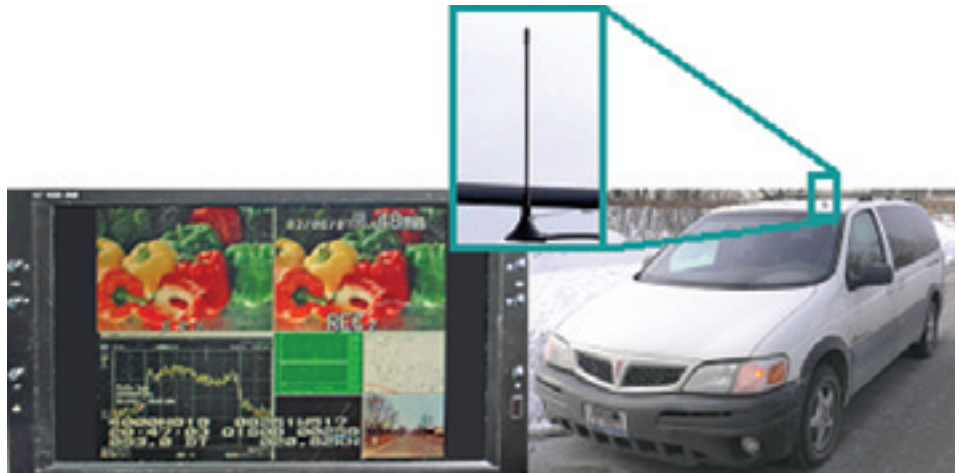
Field trials of the MPH system showed rock-solid reception in a moving vehicle with a single rooftop antenna.
