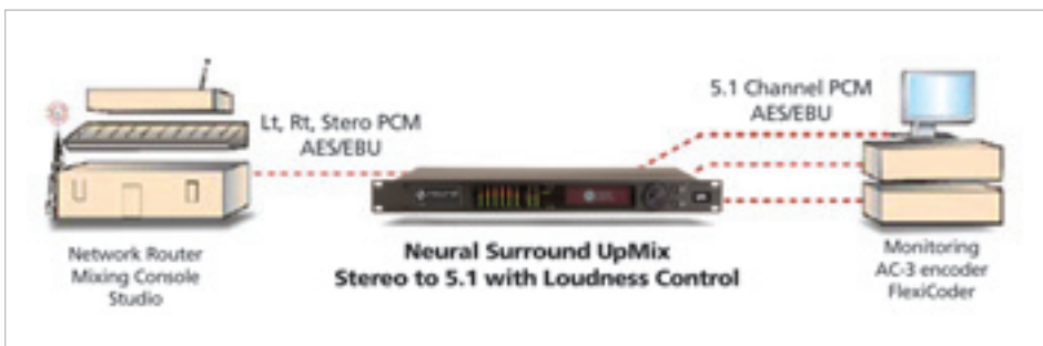
Neural-THX® Surround UpMix is commonly used for audio monitoring, and in production studios and DTV facilities.
